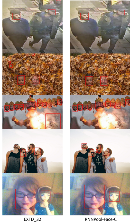
Figure 7: Comparison of performance on test images with EXTD_32 and RNNPool-Face-C. The confidence threshold is set to 0.6 for both models. The EXTD model has more false positives and misses more faces. In the first image, EXTD makes a faulty prediction at the top right. In the second image, EXTD mistakes regions in leaves for faces, while our model detects just the two correct faces. In the next image, both the models have some wrong detections, but the EXTD model detects a large bounding box that is a false positive. In the next image EXTD misses a face with an unnatural pose that our model detects. However, our model detects a face within a face which in general can be removed easily. In the next image (last row above), both the models detect the two faces, which weren't detected by the models on the left. Our model detects a slightly better bounding box than EXTD.
